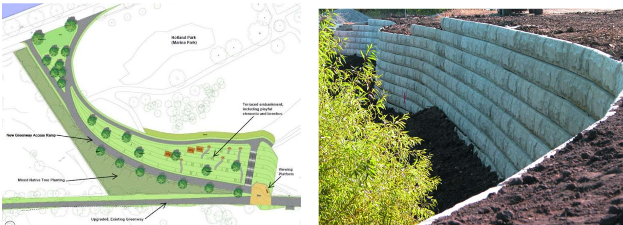
Figure 4.17: Example of landscaped ramp (left) and soil reinforcement retaining wall (right)
