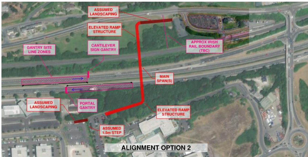
Figure 2.9: Bridge Alignment Option 2
