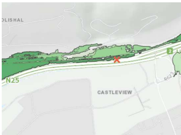
Figure 4.1: Screenshot from floodinfo.ie showing extent of potential coastal flooding at location of proposed alignment
